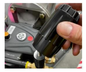
4. Remove the adjustment knob and set aside
