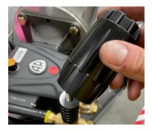
IT MAY TAKE SEVERAL TIMES OF REMOVING, ADJUSTING THE JAM NUTS, AND REINSTALLING THE KNOB BEFORE ACHIEVING THE CORRECT MAXIMUM PRESSURE SETTING FOR THE PRESSURE WASHER SYSTEM.
